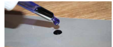
Ink test: Put a drop of ink on the anodized surface and wipe off with an absorbent cloth
