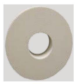
FiveP-PE felt wheels for polishing with cerium oxide subsequent to pre-polish consist of a polyester felt reinforced with adapted resins. This mixture guarantees a very high lifetime of the felt wheels and the efficient use of the used cerium oxide or alternative polishing product. The FiveP-PE felt wheels complete the polishing process for the production of the perfect high-gloss edge finish.
