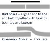
overlapped by 6mm and sealed with heat and pressure. The trailing edge is layered on top
